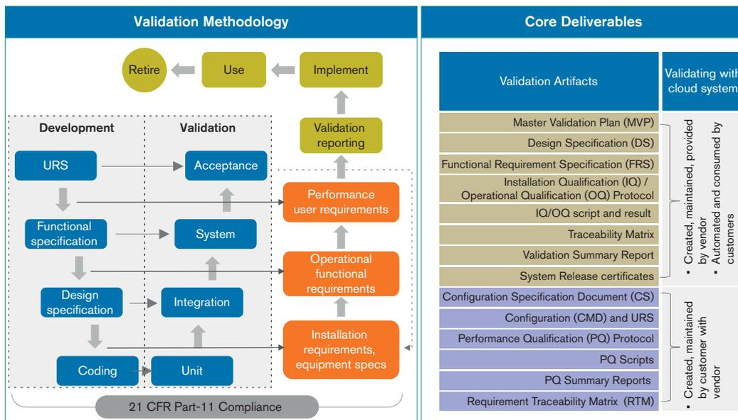
The 'V-Model' is the backbone for any CSV testing performed at Atos Syntel CoE
